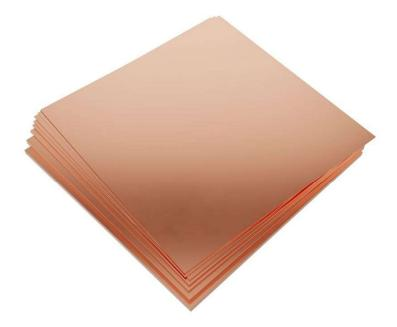
Different sets of high purity copper plates for testing Half Value Layer
