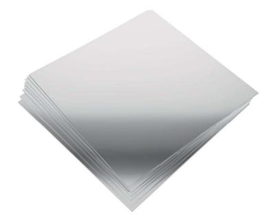
Different sets of high (99.9%) and standard (99.5%) purity aluminium plates for testing Half Value Layer
