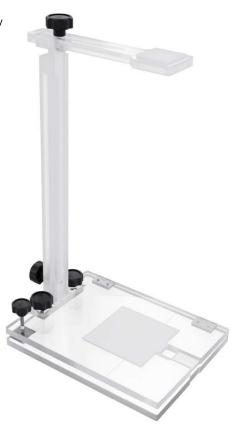
**Adjustable stand**, designed to make focal spot measuring procedures **easy to perform**, as well as **ensuring accurate results** It can also be used for the HVL measurements.
