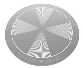
With Pro-Star test Patterns focal spot size can be determined by observing the regions of blurring which occur when the pattern is radiographed by an x-ray source of finite dimensions.
