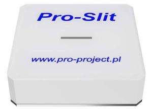
The Pro-Slit phantom is the so called **slit camera for accurate measurement of the focal spot size according to IEC.60336:2005** Its main advantages are **repeatability, accuracy and possibility to measure the size of any focal spot.** Because of the small attenuation of the outer cover this tool can also be used with dental digital detectors - detector receives enough radiation to be triggered.
