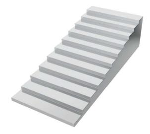
A 11 step aluminium wedge for evaluation of dynamic range of digital or film-screen systems
