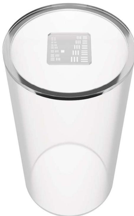
**A simple test device for the focal spot size evaluation** . It consists of a precision bar pattern placed at the end of the cylinder that provides accurate and reproducible target-to-image receptor spacing.
