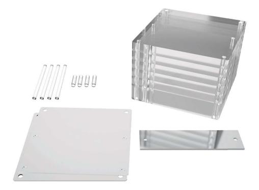
A set of acrylic and aluminium filters for testing diagnostic X-rays according to AAPM recommendations from Report No. 31"Standardized Methods for Measuring Diagnostic X-Ray Exposure". Patient-equivalent acrylic and aluminium phantoms provide the necessary attenuation between the source and AEC or ABC detectors.
