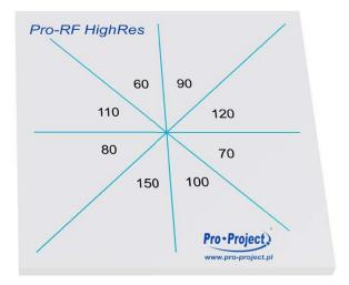
The test phantom for **evaluation of high contrast resolution of fluoroscopy system in one exposition**. It consists of eight patterns of wire mesh in a pie shape.
