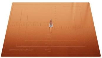
This device readily indicates a 1% or 2% misalignment at a 1 m focal-film distance (FFD), but it can be used at any FFD It consist of a flat 20 x 25 cm plate with a 14 x 18 cm pattern etched on its surface. It can also be used to check fluoroscopy alignment and collimation.
