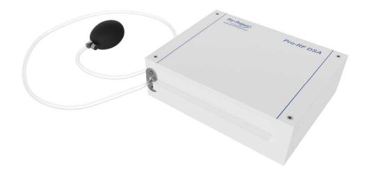
A special phantom for Quality Assurance of Digital Subtraction Angiography Equipment(DSA)o IEC 61223-3-3 and DIN 6868/Parts 8, (2007) and 54 The phantom contains a movable insert with aluminium strips to simulate blood vessels. This insert can be moved via pneumatic system from a safe distance during exposure.
