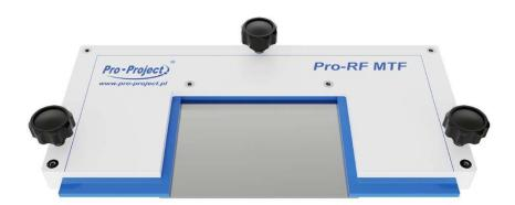
The edge test device according to IEC 62220-1 for determination of Modulation Transfer Function that consists of a tungsten plate fixed on a lead plate.
