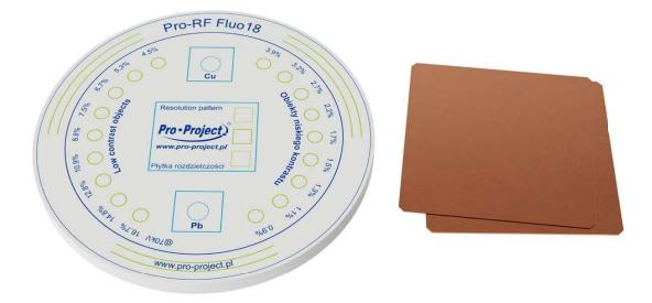
The phantom for evaluation of imaging performance of fluoroscopic systems. It allows brightness and contrast adjustments, circular geometry check (scanning linearity) plus wide-range low-contrast and high-contrast resolution evaluation. Available in two standard layouts plus any custom configuration.
