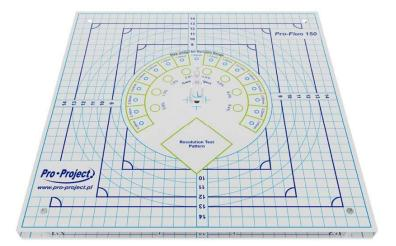
The Pro-Fluo 150 phantom is dedicated for acceptance and constancy tests of radiography and fluoroscopy equipment according to the new DIN 6868-150 standard
