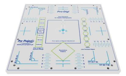
The Pro-Digi phantom is dedicated for acceptance and constancy tests of digital radiography equipment.
