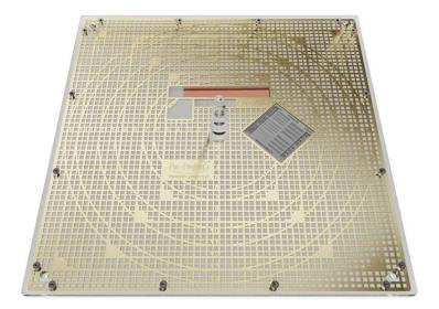
The Pro-Alpha phantom can be used for carrying out acceptance and constancy tests of conventional radiography X-Ray units.
