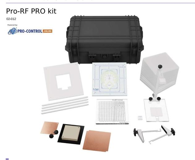
This kit is a versatile set of phantoms and software for carrying out constancy tests of radiography and fluoroscopy units. Thanks to the Pro-Control.online subscription, all tests can be quickly and effortlessly automatically analysed online and with the desktop app.
