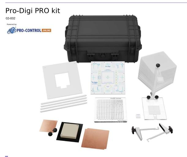
This kit is a versatile set of phantoms and software for carrying out constancy and acceptance tests of radiography x-ray units. Thanks to the Pro-Control.online subscription, all tests can be quickly and effortlessly automatically analysed online and with the desktop app.
