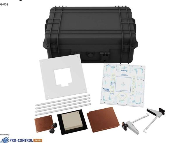
This kit is a versatile set of phantoms and software for carrying out constancy tests of radiography x-ray units. Thanks to the Pro-Control.online subscription, all tests can be quickly and effortlessly automatically analysed online and with the desktop app.
