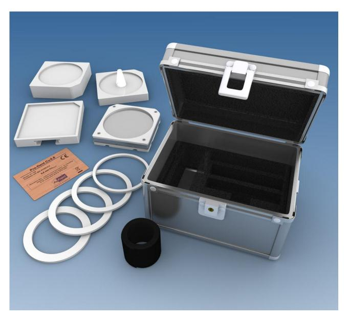
The Pro-Dent set is a universal set of phantoms for carrying out constancy and acceptance tests of conventional and digital dental X-ray units (intra-oral, panoramic and cephalometric).
