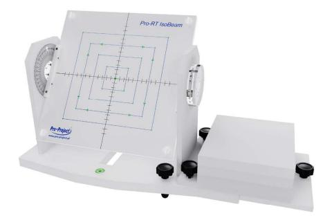
This is a multifunctional, precision quality assurance tool for daily, weekly or monthly quality assessments of all mechanical and geometrical treatment parameters of linear accelerators or teletherapy units
