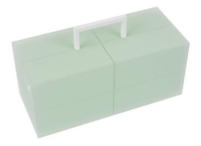
Rectangular MRI phantom simulating attenuation of the human spine.
