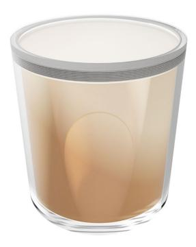
This stability (agar) phantom consists of a cylindrical phantom and agar material inside. Using this phantom a Signal to Noise Ratio, Signal Fluctuation to Noise Ratio, drift, and other imaging measures over a 100-volume or 200-volume fMRI scan can be performed. The agar phantom has characteristics similar to the T2 measures of a human head, but provides no change in signal. The T1 and T2 characteristics of the agar phantom at 3T are ~900 ms T1 and 30 ms T2.
