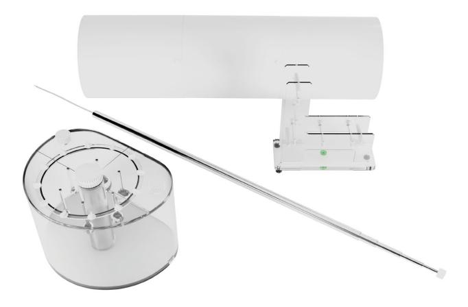
This kit is a versatile set of phantoms and software for carrying out tests accoring to NEMA NU 2 standard on PET devices. Recommended for use in the evaluation of reconstructed image quality in whole body PET imaging. It can be used to measure the effects of dead-time and the effects of random events generated at different levels of activity of the line source, characterize the widths of the reconstructed image point spread functions (PSF) of compact radioactive sources.
