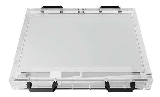
The Pro-NM AutoFlood is dedicated for weekly inhomogeneity and sensitivity control and acquisition of correction matrices, according to revised Guideline on Radiation Protection in Medicine. Regarding its dimensions the Pro-NM AutoFlood corresponds to DIN 6855, Part 2. It contains a mixing system with built-in pump. Due to its special composite design, deformation of the measuring areas is avoided by permanent water contact.
