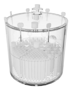
The phantom for high resolution NM and PET systems performance evaluation (collimator, artifacts, calibration, reconstruction parameters).
