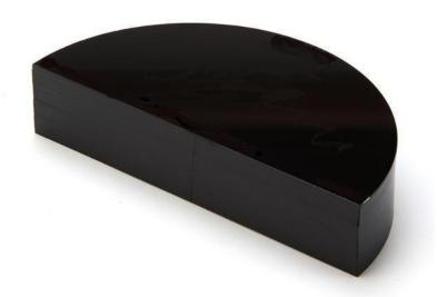
A breast tissue simulating test object designed to be used to compare image quality between different exposure parameters within a single system or across different breast tomosynthesis systems.
