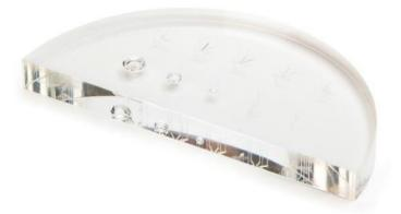
Phantom into which liquids (e.g. saline or BMF + contrast agent) can be injected so that contrast agent studies can be performed. Includes spherical voids of 1, 2, 5, 10, 15 mm diameter and fibrous features with a range of sizes. Includes syringe and needle type bd micro-fine 0.5 ml u-100 insulin syringe.
