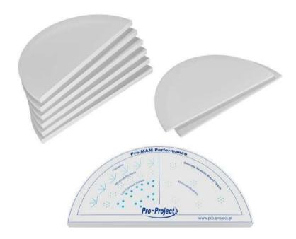
The phantom designed to be used for routine quick and ongoing checks of imaging performance of mammography systems. It allows evaluating particularly those aspects which are most liable to deterioration.
