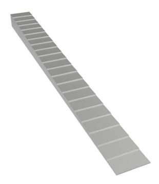
**21 step aluminium wedge** for determination of **the dose reproducibility and sensitometric curve shape, speed and mid-gradient** of mammography X-ray film.
