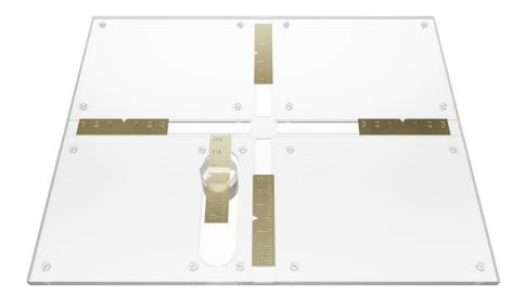
This test device was developed to provide the user with a convenient, quick and accurate way of testing collimation of mammography units. It is very simple to use. Instead of using all those hard-to-find coins, you only use our test tool.
