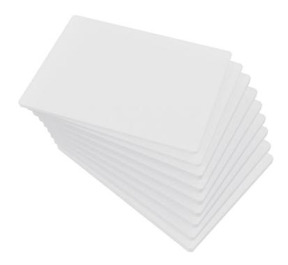
Set of acrylic plates for testing Automated Exposure Control of mammography systems.
