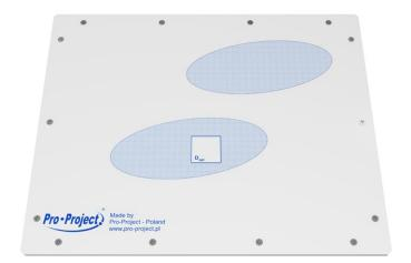
Test grid for testing mammography-cassette film-screen contact.
