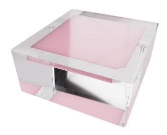
The phantom can test the performance of a mammographic system and its ability to image small structures similar to those found clinically: calcifications, fibrous calcifications in ducts and tumor masses.
