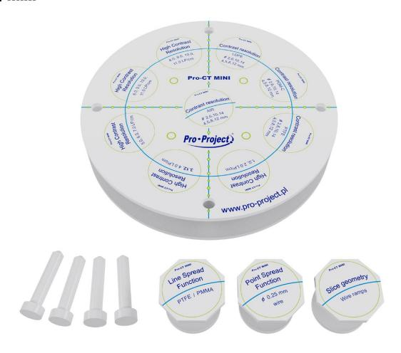
The Pro-CT MINI phantom is a compact CT image quality testing solution. When connected with Pro-CT Dose it may be used for carrying out acceptance and constancy tests of computed tomography systems according to IEC 61223-3-5 and the AAPM (American Association of Physicists in Medicine) guidelines. This phantom consists of a module 16cm in diameter with positioning aids and recesses for test modules.
