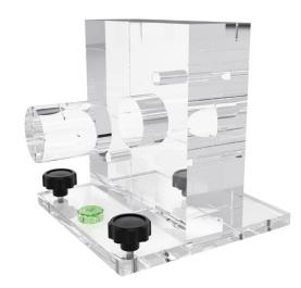
This phantom can be used to check the alignment of the internal and external lasers to the radiographic center of CT and PET/CT units and to verify lateral gantry angle. It can also be used with accelerator units to check vertical and lateral gantry angles, laser alignment and vertical table movement.
