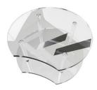
• three aluminum strips, 0.5 mm thick and 25 mm wide angled at 45°, positioned at the centre and aligned vertically
